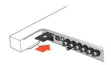
4 - The new configuration will be read automatically by your Devialet on insertion of the SD card. There is no need to restart the device.
