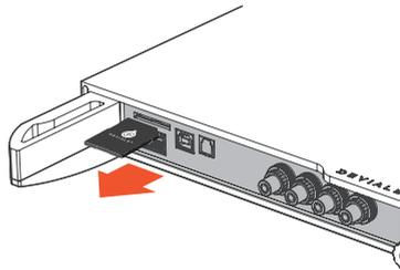
2 - Once the update file has been downloaded from the [www.devialet.com](http://www.devialet.com) website and saved to your SD card, reinsert the card in the card reader of your Devialet (without write protection).
