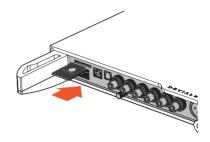
4 - The new configuration will be read automatically by your Devialet on insertion of the SD card. There is no need to restart the device.
